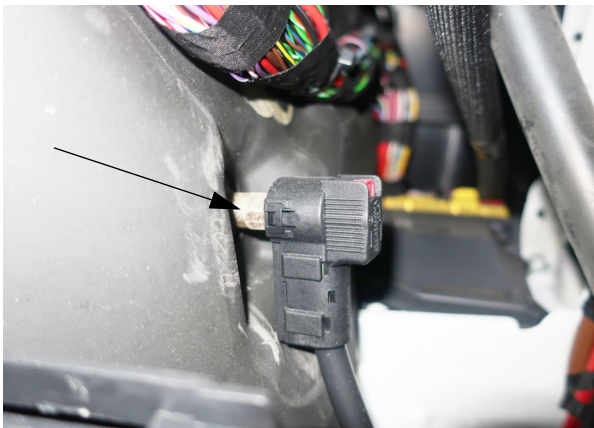
Chassis Battery Connector (Located to the right of the accelerator pedal behind access panel)
