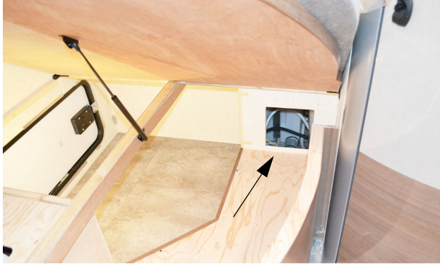
Water Pump (Located behind removable access panel below bed) -Model 24J shown
